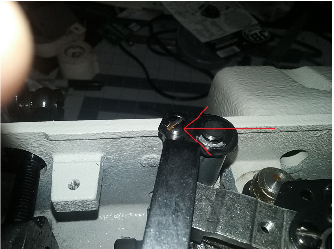
Finally adjust bobbin hook with this screw.
